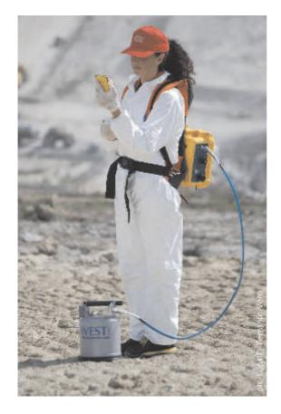
Such procedures involve geo-referenced flux measurements, on a regular grid, of the entire landfill body.
